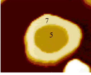
FIG. 1. (Color online) 281 \times 205 nm 2 STM image of the Pb islands grown on Si(111)-( 7 \times 7 ) surface. The numbers indicate the height of the different areas and a smooth bilayer ring has formed.
